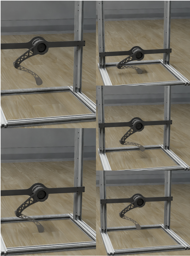
Fig. 3. Simulation of the robotic leg in the Isaac environment, illustrating the leg model during different phases of locomotion.
